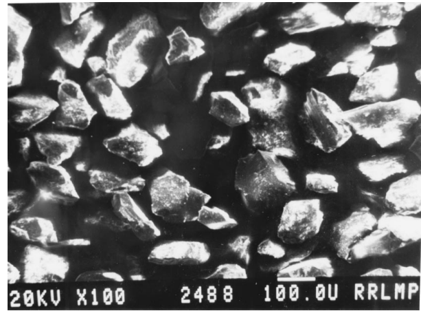
Figure 2 SEM micrograph of granite particles.
